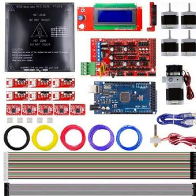
Gambar 2. 7 *Electronics Control 3D printer* (Zhao et al., 2020)
