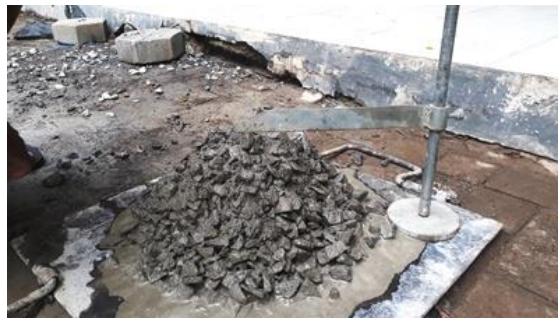
Gambar 4. 11 Uji Slump Beton Normal
