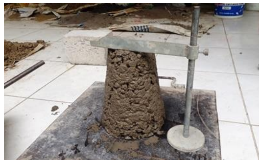
Gambar 4. 12 Uji Slump Beton Campuran 10% Fly Ash + 7,5% Lumpur
