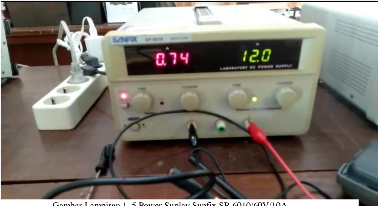
Gambar Lampiran 1. 5 Power Suplay Sunfix SP-6010/60V/10A
