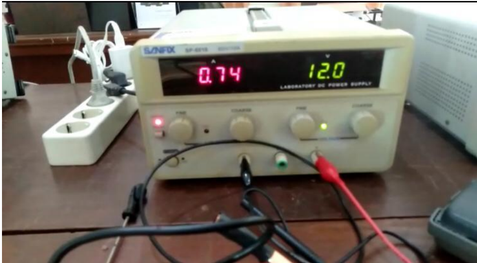
Gambar 4. 1 Power Suplay Sanfix SP-6010/60V/10A
