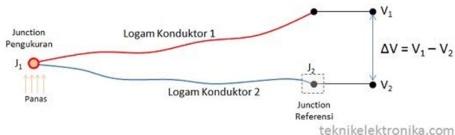
Gambar 2.6 Prinsip Thermocouple (Sensor suhu)
