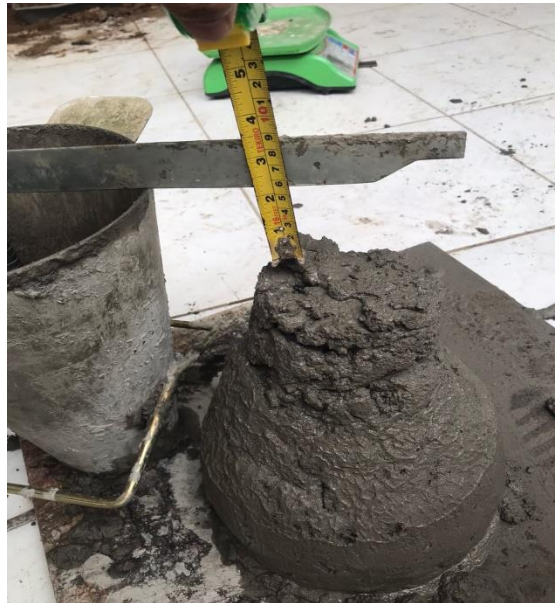
Gambar 4.7 Uji Slump Test
