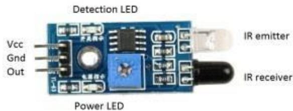
Gambar 2.2 IR Obstacle Sensor
