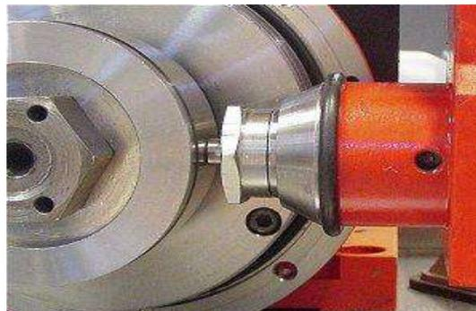
Gambar 2.14 Tribometer *pin on ring*
