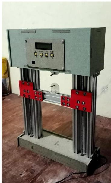
Gambar 4.1 Alat Uji Tarik Mini Berbasis Arduino
